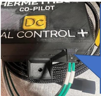
Step 6d: Molex terminal. Plug the harness from your roaster here. NOTE: one of the 4 pins is a different shape to prevent plugging it in incorrectly. Do not force the plug if it doesn't seem to fit. When properly inserted, the green wires will be facing you as pictured.
