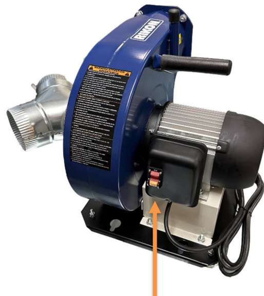
Exhaust Blower switch
