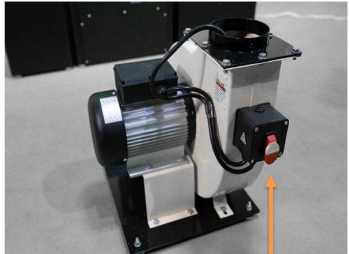
Exhaust Blower switch
