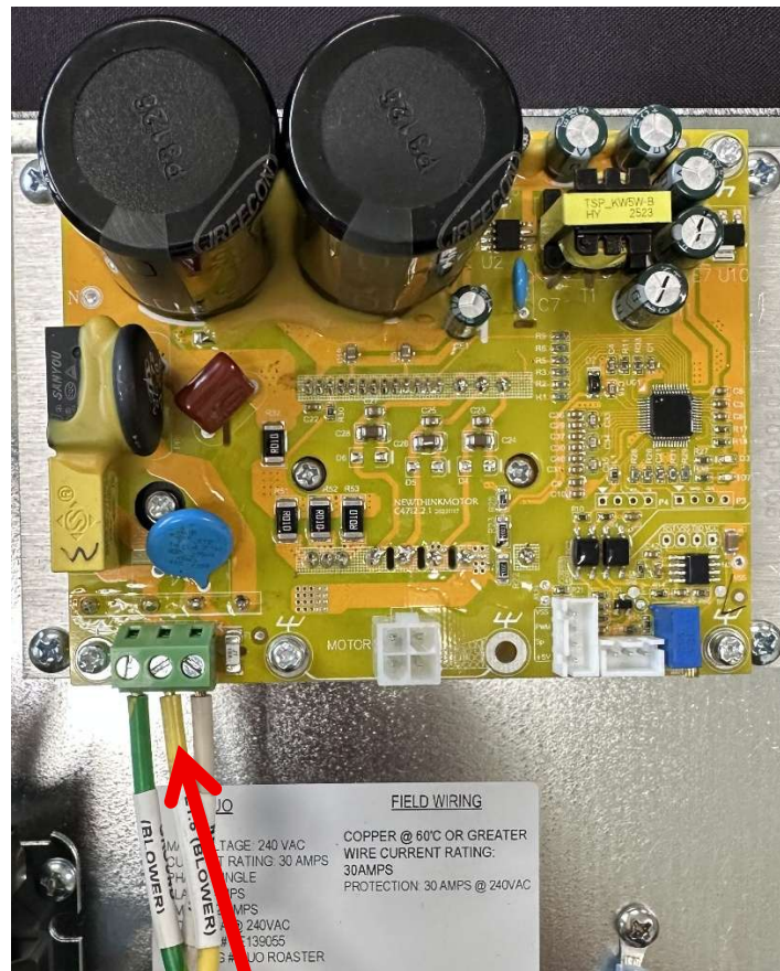
Figure 1.6 — Loft Motor Controller
