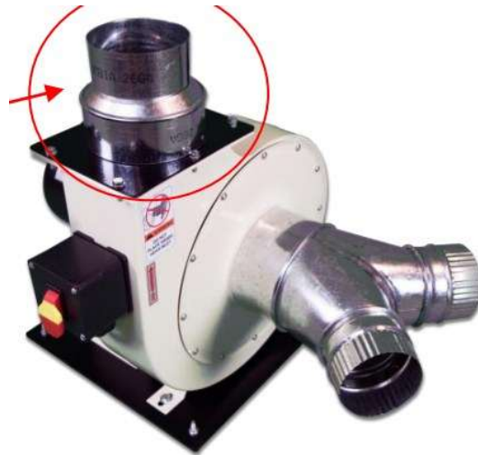
5"-to-4" reducer on the blower discharge
