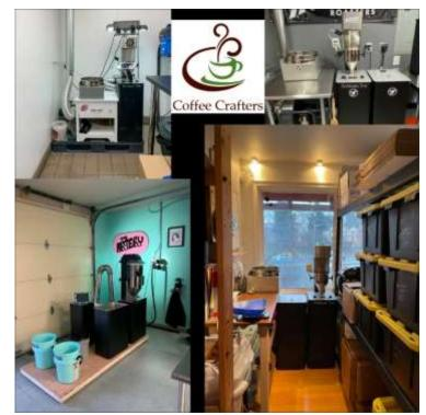
If you are roasting inside, you must consider where your exhaust duct will go. This system vents just like a clothes dryer and you must have access to clean the exhaust ducts. Setting up your roaster near an outside wall works best. Shorter exhaust runs make for more efficient venting and cooling. If you have questions about installation call the roaster manufacturer so you can make an informed decision.
