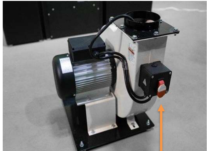
Exhaust Blower switch
