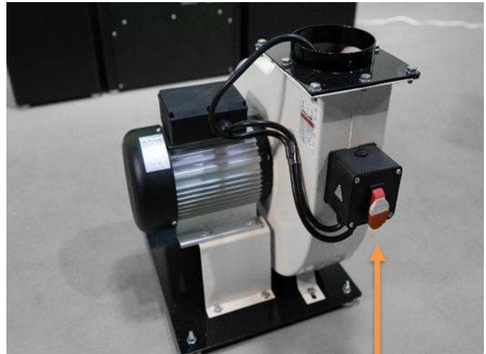
Exhaust Blower switch
