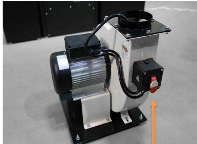
Exhaust Blower switch
